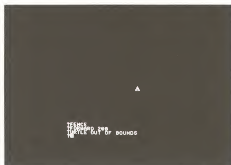
Figure 2.29: The message given by Logo when the turtle is commanded to move too far in FENCE mode.
