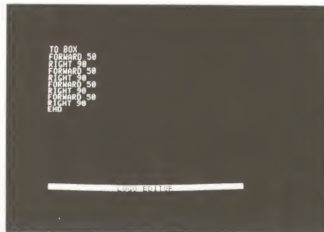
Figure 4.4: The screen as it appears after the BOX procedure has been typed in edit mode.
