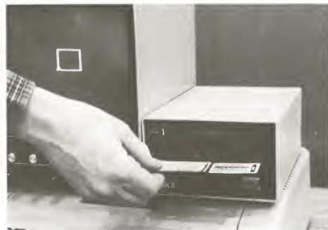
Figure 4.11: Inserting the Logo work disk into the disk drive.
